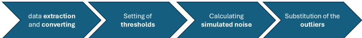
Figure 6: Visualized Steps for the Data preparation for the AE-Training.
